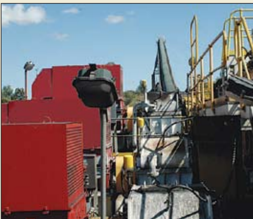
Oaky North ramp conveyor with 3 x Dodge 1120K CSTs with 1MW motors.
